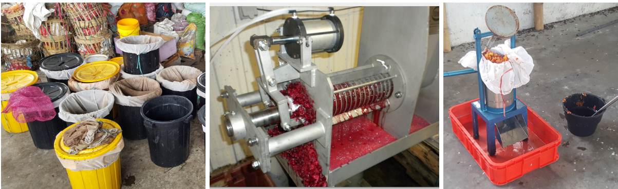
Figure 20: Different dewatering methods: passive dewatering by gravity (left), screw press (middle), cider press (right), (Photo screw press: Vincent Corporation)
