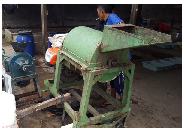
Figure 15: Hammer mill for waste pre-processing
