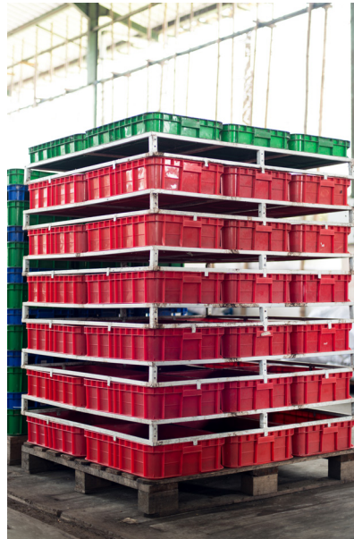
A stack of larveros. The metal frames allow ventilation and thus help water to evaporate from the waste (T1-2)
