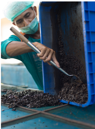
Separation of larvae and wet residue on the screen (H1-5)
