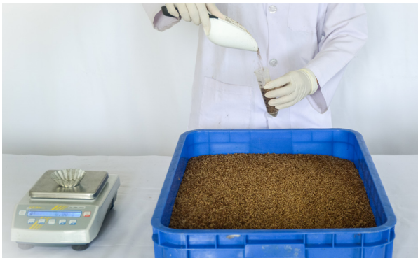
After mixing to homogenize the purified section of 5-DOL, a random scoop is taken ( R6-3 )
