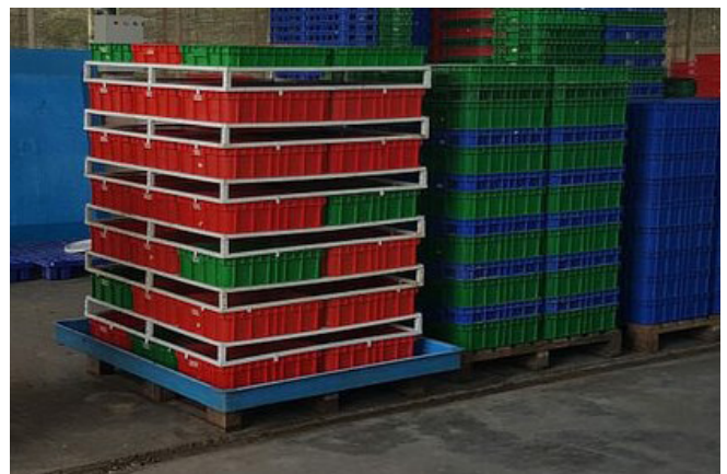
Figure 16: Stack of larveros with ventilation frames in-between levels
