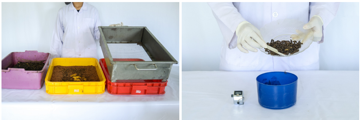
4. Prepupae-coco peat-mix from transfer containers and sieve (mesh size 3mm) 5. Click counter , plate and soft tweezers
