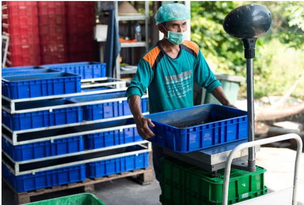
A larvero is weighed with the bulk scale before its content is emptied onto the harvesting screen (H1-3)
