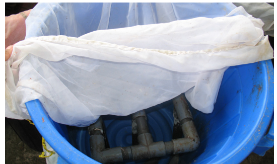
The plastic frame inside the bucket keeps the cloth and thus the waste away from the drained water ( W2-1 )
